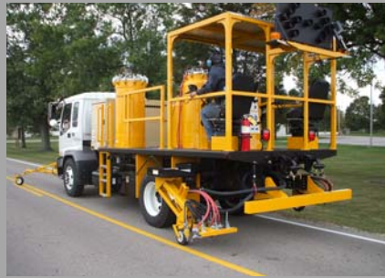
Simultaneous center & edgeline striping
