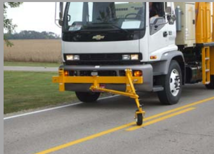
Hydraulic pointer assembly
