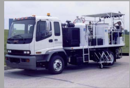
Paint vats standard equipment on WV3-AL
