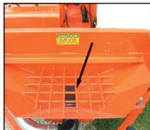
The hopper receives aggregate from the dump truck.
