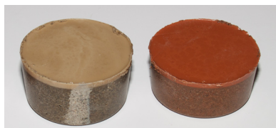
Roadware MatchCrete Concrete Mender™ with sand on the left and with sand and Solomon brand color on the right.
