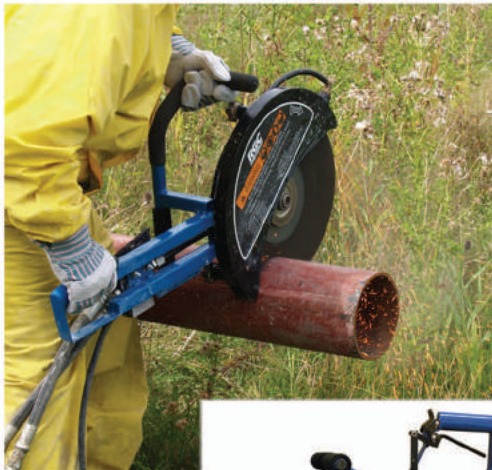
S16 HydraSaw Cutting Steel Pipe with an Abrasive Blade
