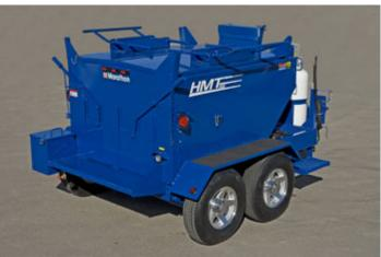
The HMT8000 is a heavy duty, fully insulated asphalt hauler complete with heated tool chamber and liquid asphalt compartment. This unit meets all the requirements to keep your patch crew productive while maintaining the proper temperature of the patching material.
