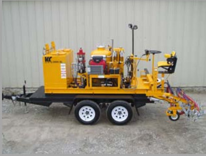
Self contained center & edgeline striper
