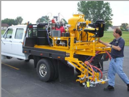
Optional drums & hydraulic power steer
