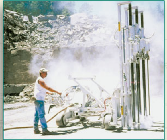
A-3 Vertical Quarry drill with a 144" drill depth.
