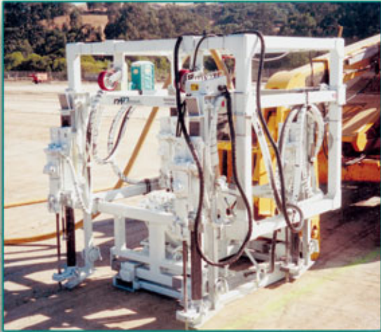
A-4 Vertical Equipment mounted drill that can drill in five different configurations.
