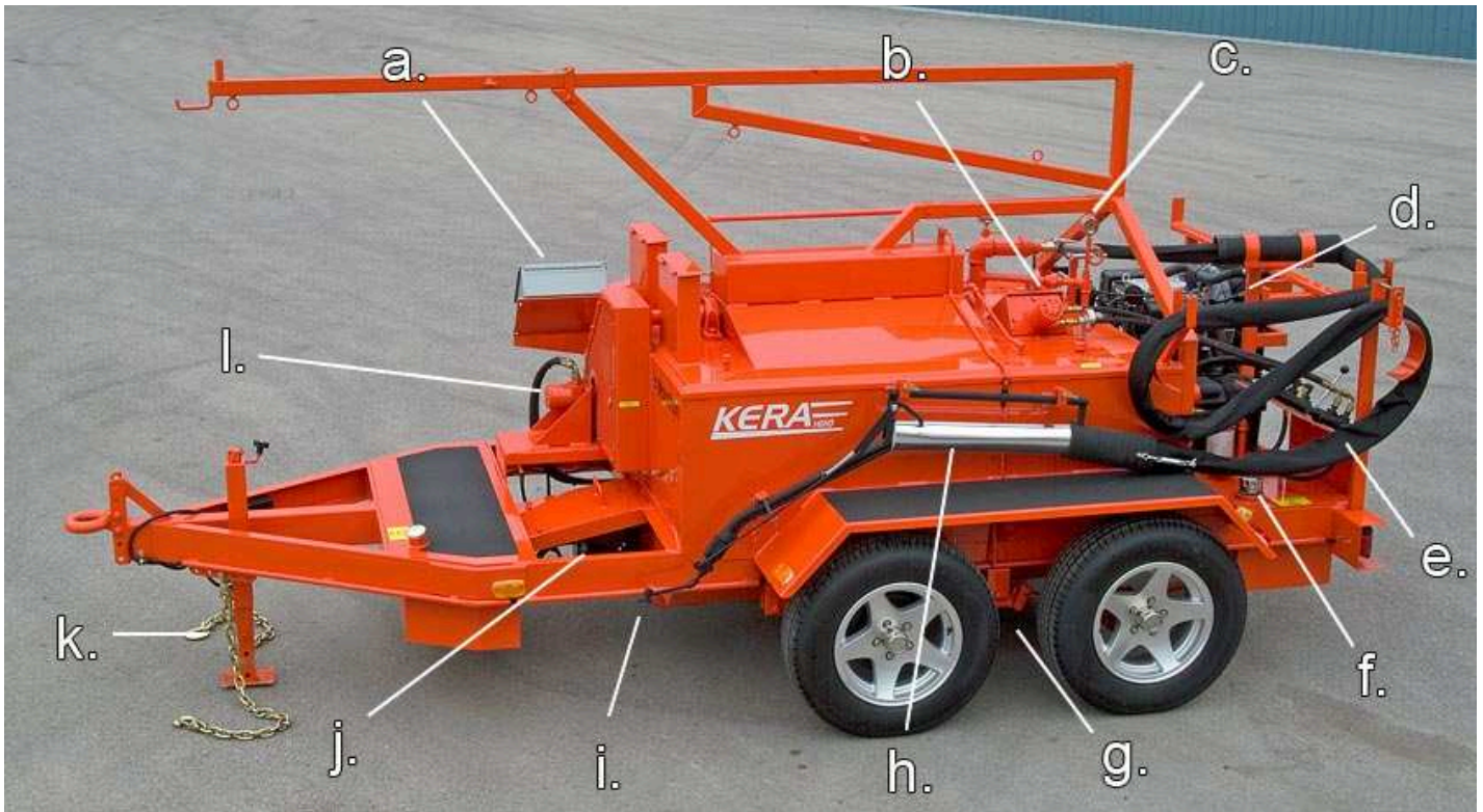
Hose boom keeps hose off of ground to improve longevity and reduce operator fatigue.
